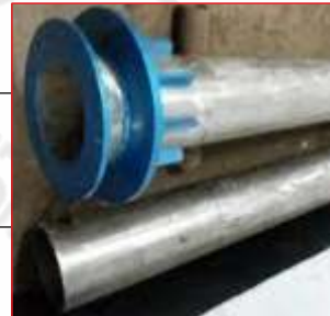
CENTRAL BURNER PIPE (CB Pipe)
